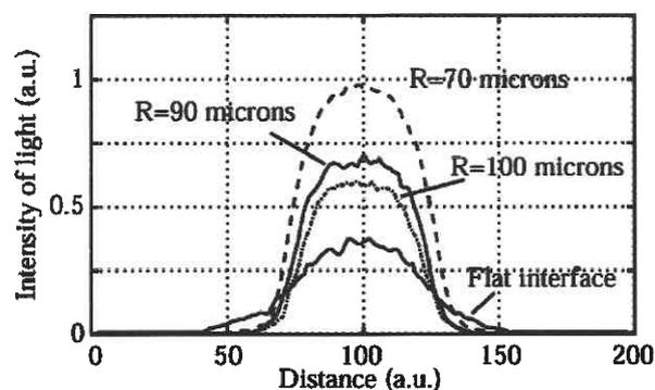
Fig. 2 Effect of the PDMS lens on the fluorescent light emission from the dye
