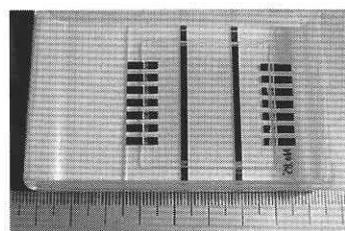
b) The OLED fabricated on glass substrate, with the encapsulation system
