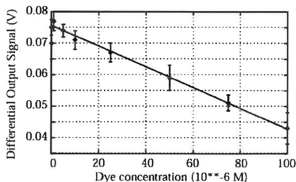
Fig. 6 Output signal of PMT versus the concentration of fluorescent dye
