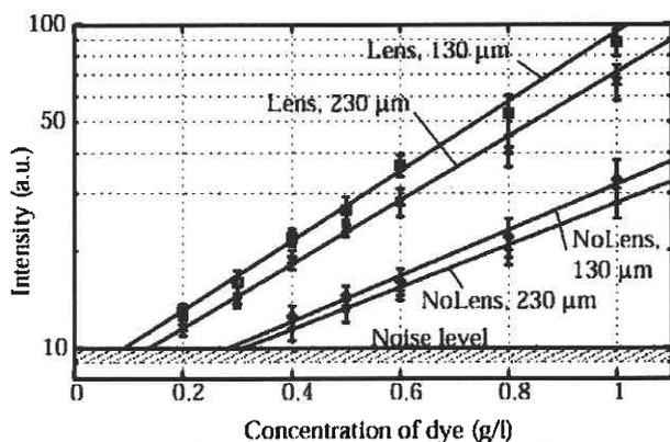
Fig. 3 Response of the labeled solution flowing inside a microchannel to an excitation by an optical fiber: comparison of the design with lens ( $70\ \mu\text{m}$  curvature radius lens) and without any lens (flat air-PDMS interface). The distance between the end of the fiber and the microfluidic channel are indicated in the graph.
