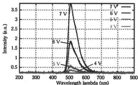
Fig. 5 Optical characterization of the OLED fabricated on a glass substrate: spectrum of the light emitted by this organic diode depending on the input voltage
