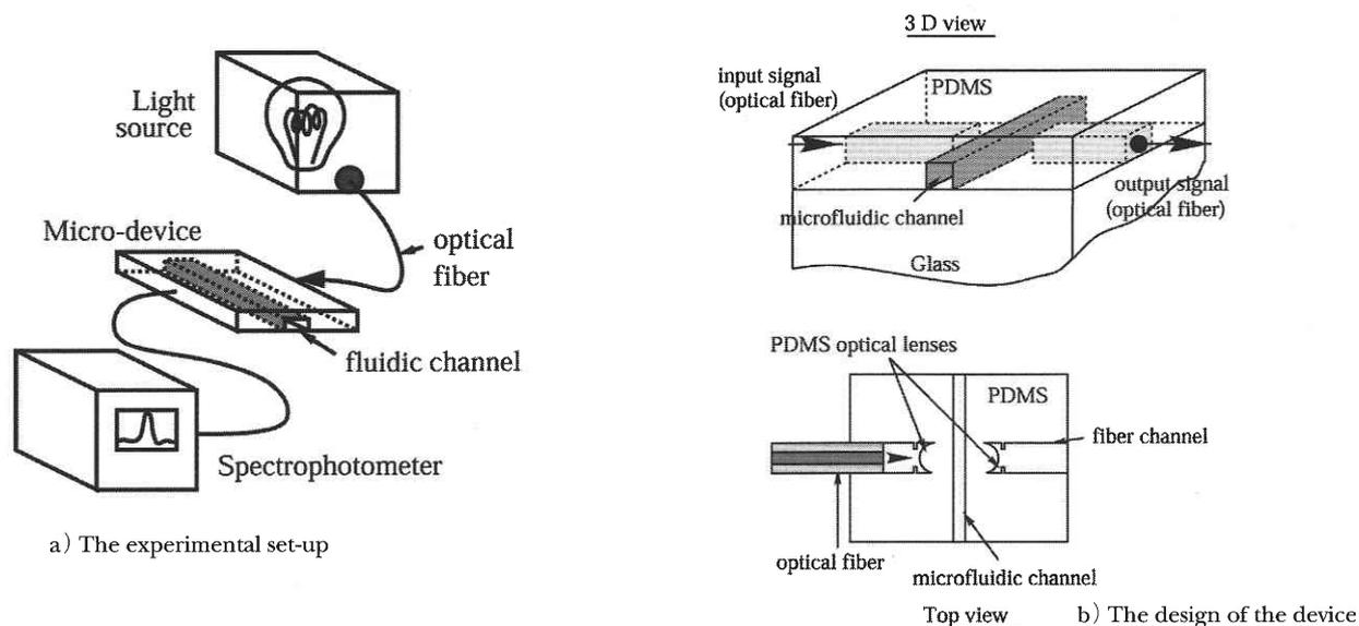
Fig. 1 The portable device using optical fibers
