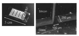
Figure 3 Photograph of the microfluidic device and close-up view of the high aspect-ratio silicon microelectrodes.
