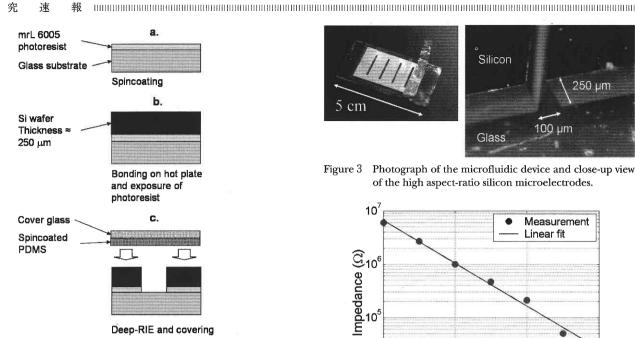
Figure 2 Fabrication process of the microelectrodes.
