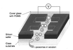
Figure 1 Schematic view of the device and protocol to fuse liposomes. Various gaps of electrodes have been designed. 1) Liposomes are aligned along the electric field lines by AC voltage. 2) DC pulses inducing high electric field perform the breakdown of membranes. 3) These membranes reconnect to form a hybrid vesicle.
