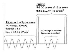
Figure 5 Voltage waveform for the electrofusion of liposomes.
