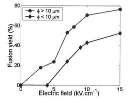
Figure 7 Experimental fusion yield as a function of the applied electric field for liposome diameters  $\phi$  larger and smaller than  $10\mu$ m.
