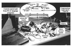
Fig. 9: Test bench of the micro conveyance system
