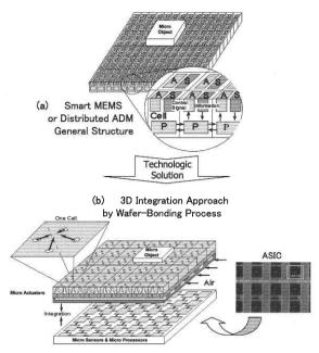
Fig. 11: Smart MEMS design approach
