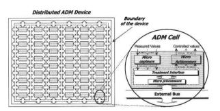
Fig. 1: Structure of distributed ADM device
