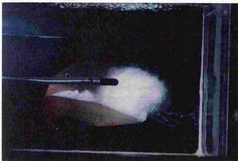
Fig. 6.3: Cavity appearance, KT section, 8^\circ , 12 m/sec., \sigma_B = 1.25
