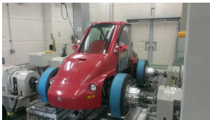
Fig. 33: Real Car Simulation Bench
