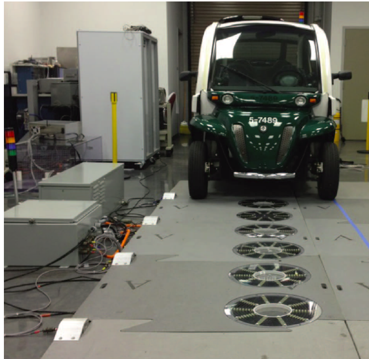
Fig. 2: Experiment on Dynamic Wireless Power Transfer at Oak Ridge National Laboratory.[13]
