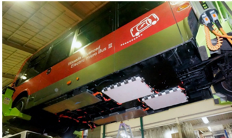
Fig. 3: 22 kW receivers with geometrical position shift.[17]
