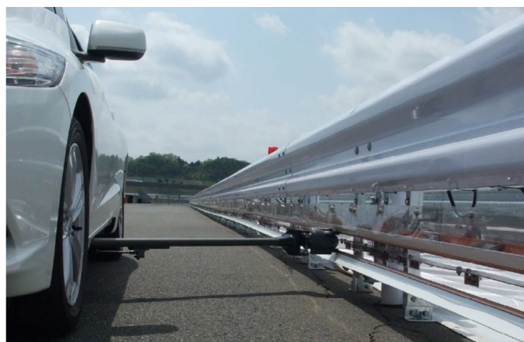
Fig. 1: Dynamic Charging Lane & Vehicle.[8]
