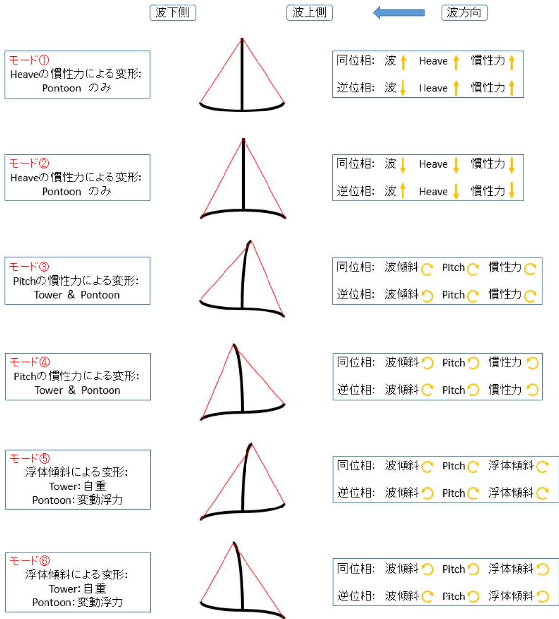
Figure 6-17 Deformation Mode of Tower and Pontoon
