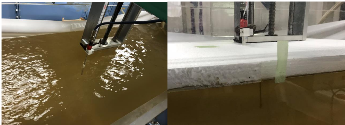
Figure 4.29 - Scenes of velocity profile measurement by an anemometer in a circulating water channel
