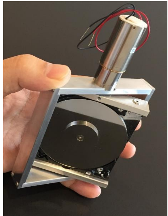
Fig. 10 Small model of gyro generator
