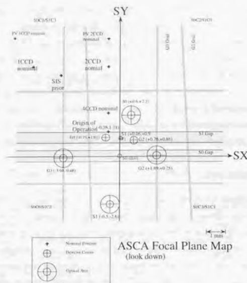
Figure 4.6: Alignment of the detectors. The optical axes and detector centers of SIS0, SIS1, GIS2, and GIS3 are shown. Nominal positions for various observation modes are also plotted in the figure.
