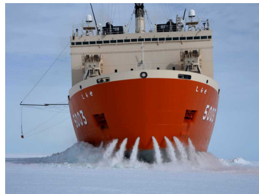
Fig. 1 Water flushing system[1]
