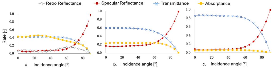
Fig 2. Variations of reflectance, transmittance and absorptance with incidence angles to window surface. (a) RRF; (b) HSF; (c) SFG
