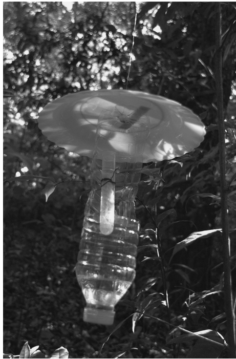
Fig. 2. Ethanol-baited trap modified from a 550 ml soda bottle; 95% ethanol was put into a conical tube suspended inside the trap. A cotton rope was placed into the tube as a dispenser. Propylene glycol was put in the bottom of the bottle to kill and preserve insects. A plastic dish was used as a roof to prevent entry of rain.
