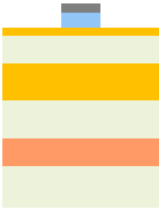
(g) Dry etch \text{SiO}_2
