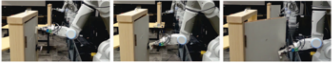
Figure 2.14: Two robots learning to open doors using asynchronous NAF. The final policy learned with two workers could achieve a 100% success rate on the task across 20 consecutive trials [31] .
