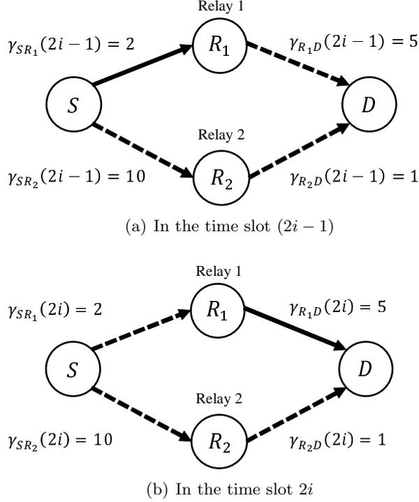
Figure 2.1: An example of the BRS with  $K = 2$  relay nodes, where solid lines represent the link selected for packet transmission, while dashed lines represent the link not selected for packet transmission.
