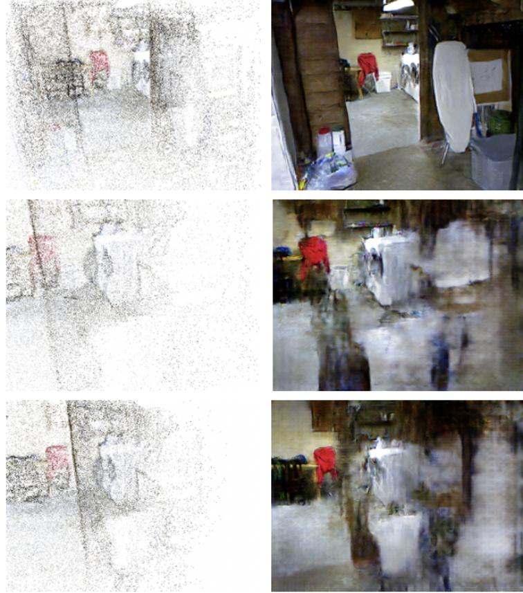
Figure 5.3: Samples of failure cases. Image pairs of point cloud projections (left) and synthesized results (right). First row: original viewpoint; Second row: virtual viewpoint generated by a translation offset \{-2,0,-4\} ; Third row: virtual viewpoint by a translation offset \{-2,0,-2\} . It is clear that poor reconstruction and strong artifacts are found in areas with fewer projected points.
