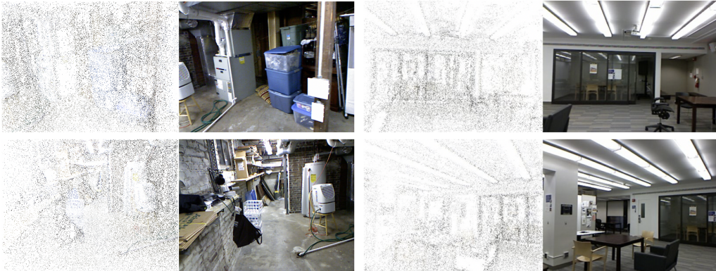
Figure 3.1: The illustration of real images with corresponding point cloud projections. The sparse point cloud with 54,665 vertices is generated from Structure-from-Motion. It could be projected into arbitrary viewpoints with specific camera parameters.
