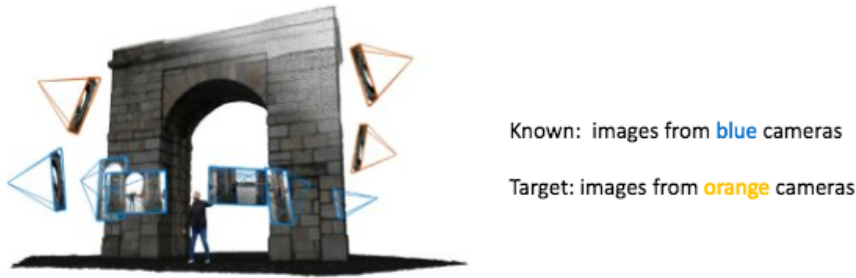
Figure 1.1: Novel view synthesis [Alj17]. The problem setting is that for one scene, if we have a sparse set of images from blue cameras, we would like to get rendering of other virtual views from orange cameras.
