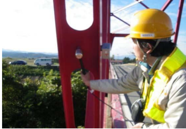
Figure 2-1 Hammer test on a truss bridge [8]
