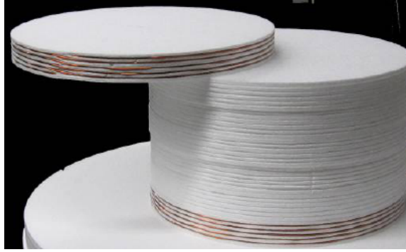
(a) Experimental setup to investigate transmission characteristics vs. antenna misalignment
