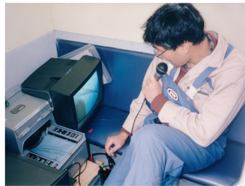
Fig. 9. Photos showing video camera system for sea-truthing in Akkeshi Bay, east Hokkaido. Underwater video camera is lowered from the boat (left photo). An observer monitors bottom features by the display in the cabin (right photo).
