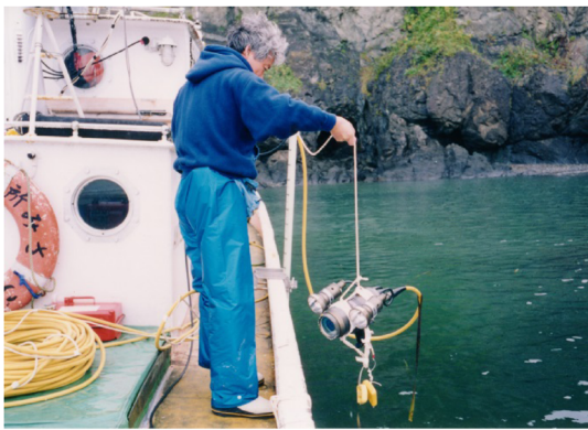
Fig. 9. Photos showing video camera system for sea-truthing in Akkeshi Bay, east Hokkaido. Underwater video camera is lowered from the boat (left photo). An observer monitors bottom features by the display in the cabin (right photo).
