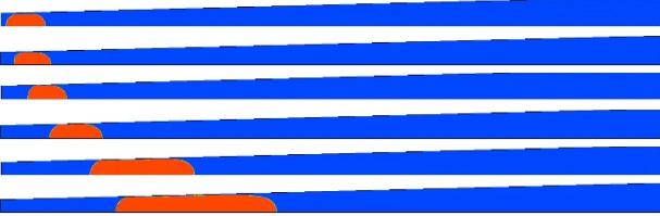
Fig. 10 Growth of bubble during flow boiling
