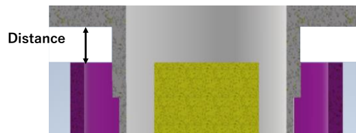
Fig 4-3 Definition of the distance between yoke and coil
