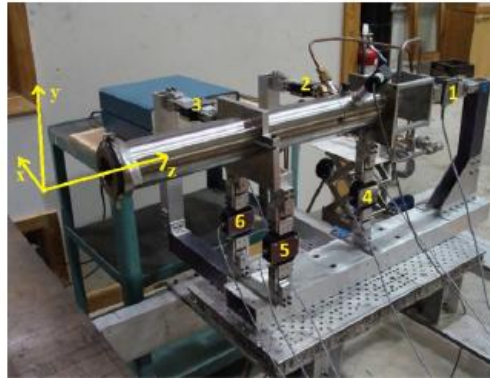
Fig 1-8 6 DOF thrust stand for hybrid rockets [36]
