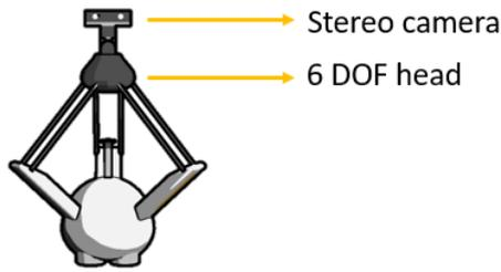
**Figure 3: Construction of 6 DOF robot RT-Telbee**
