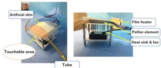
**Figure 7: New surrogate with a cooling module**
