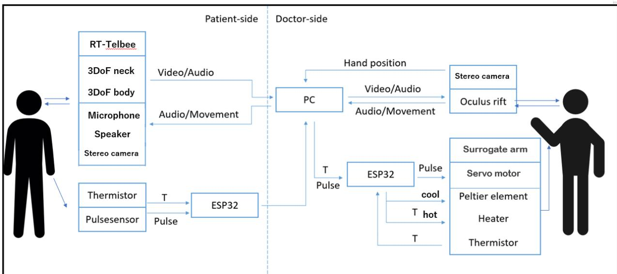
Figure 1 : System data diagram
