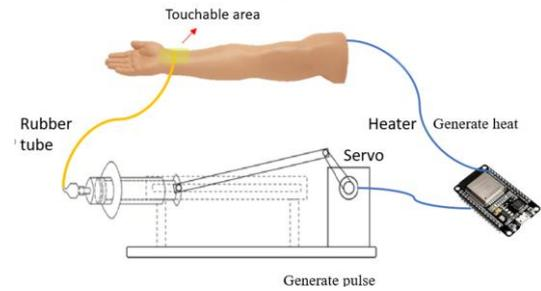
**Figure 6: Mechanism of the reproduction system**
