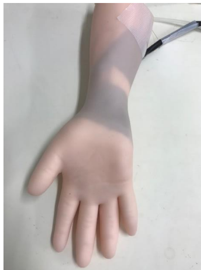
Figure 2.4-4: Silicone rubber wrapped dummy arm
