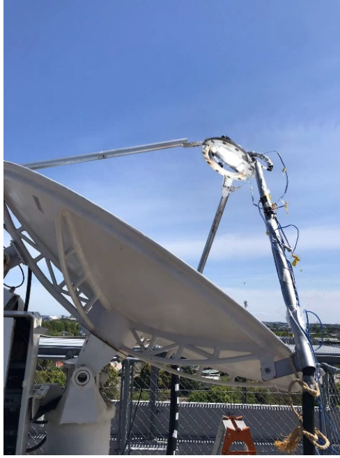
Fig.3.1: Scheme of the parabolic dish concentrator of HCPTV system
