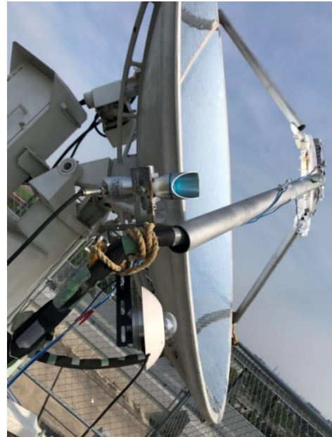
Fig.2.2: Pyranometer for recording solar radiation
