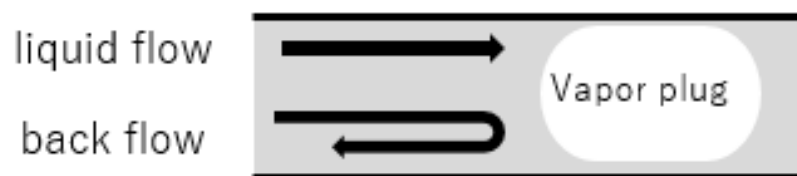
Fig.1.11: Reverse flow in micro-channel
