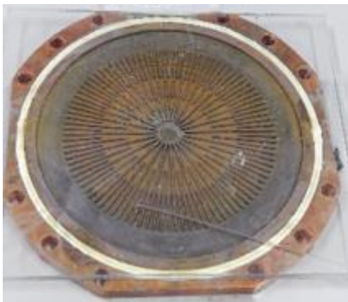
Fig. 3 Radial expanding minichannel heat sink used in this study.
