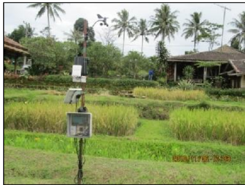
Installed Weather Station
