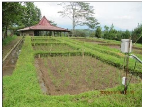
SRI paddy plots are monitored by FieldRouter
