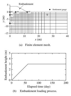
Figure 3. Setup of numerical simulation.
