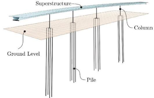
Figure 2. Bridge model, perspective view
