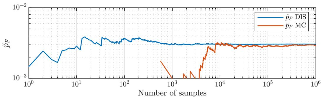
Figure 3. Evolution of failure probability estimator calculated by means of Directional Importance Sampling (DIS) and Monte Carlo Simulation (MCS)
