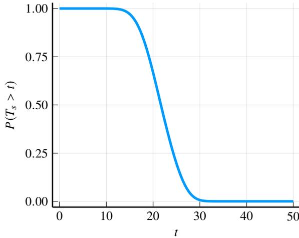
Figure 4. Reliability of the offshore jacket structure without inspection or maintenance.
