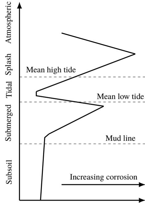
Figure 1. Relative thickness loss in different corrosion zones.
