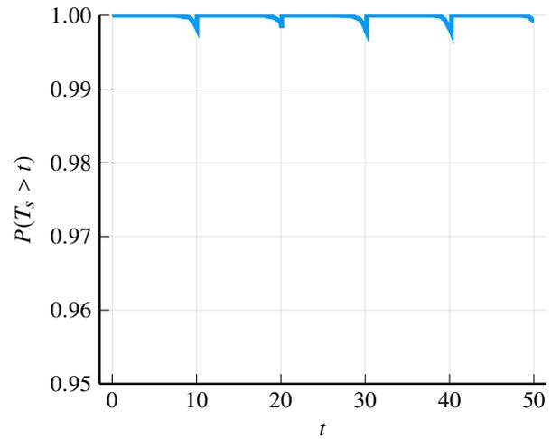
Figure 5. Reliability of the offshore jacket structure with optimized maintenance intervals.
