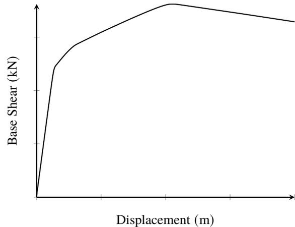
Figure 3. Typical pushover curve showing base shear over lateral displacements
