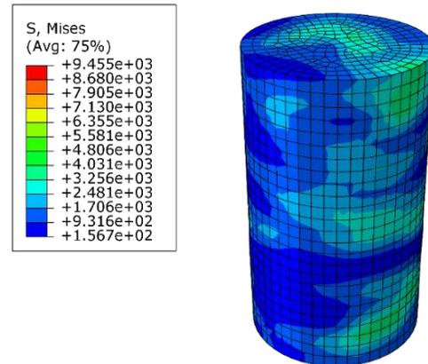
Figure 6. Finite element analysis results of cement-treated column.
