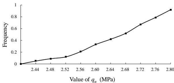
Figure 8. Cumulative distribution function graph of unconfined compressive strength.
