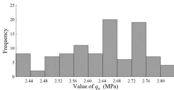
Figure 7. Histogram of frequency distribution of unconfined compressive strength.
