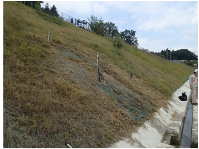
Photo 1. Field monitoring system at the target slope.
