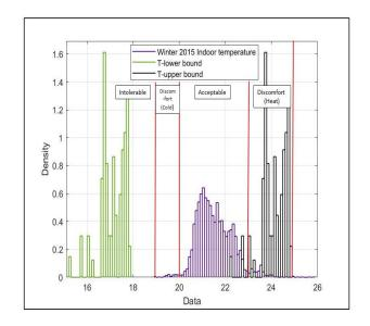
Figure 2. Indoor temperature analysis for example building (HUB) during Winter 2015.
