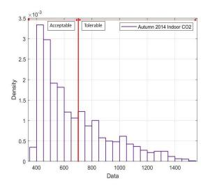
Figure 3. Indoor CO<sub>2</sub> analysis for the HUB during Autumn 2014.
