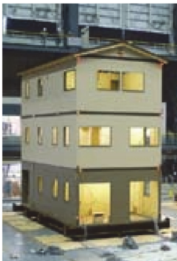
Figure 1. Specimen of wooden house (NIED 2020).
