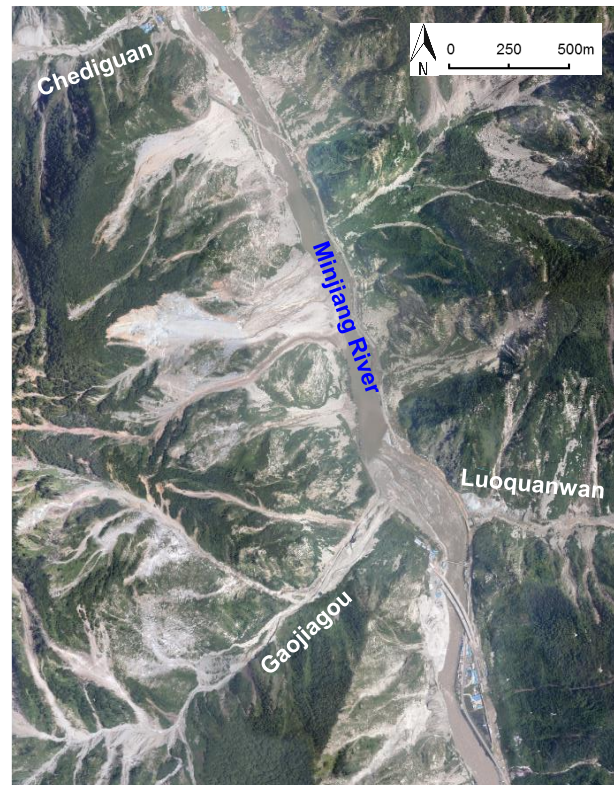
Figure 15. Debris flows on 3 July 2011 rainstorm, which largely blocked the Minjiang River and damaged G213.
