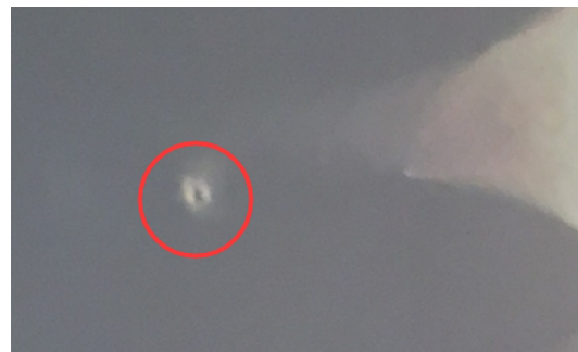
(b) Burn mark on CNT@BNNT film.
