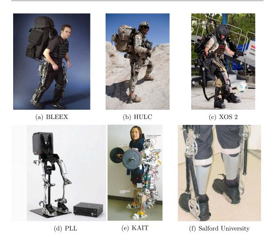
Figure 1.1: Power assist robots designed to increase humans performances such as muscle strength and endurance
