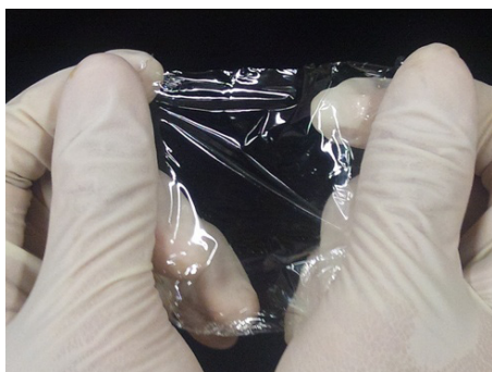
Figure 7.2. A film of poly(vinyl acetate- alt -CO) prepared by cast processing.
