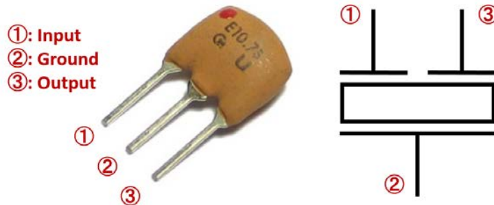
Figure 4.19 Image of 10.7MHz ceramic filter used in APT receiver, its symbol in circuit diagram and corresponding pin allocation
