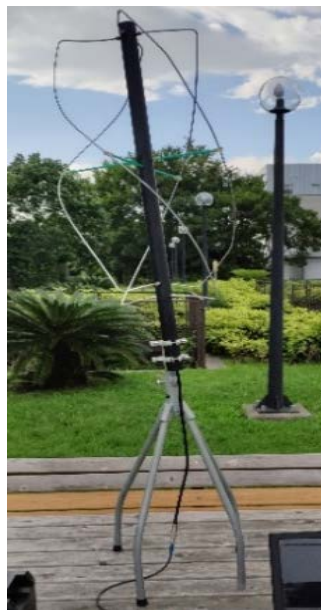
Figure 3.2: QFH antenna used in receiving APT at Kashiwa campus
