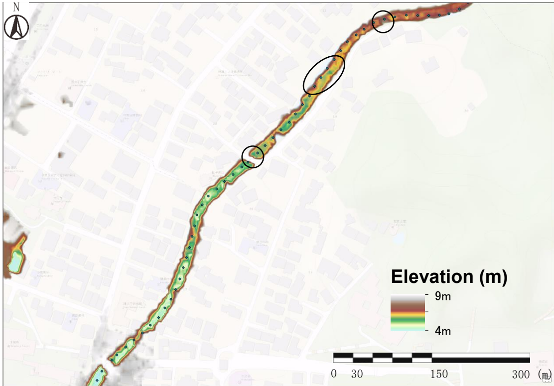
Figure 3-6D. The elevation color map of 1310m-1800m. The circles indicate the points of bridges and roads which should be removed.
