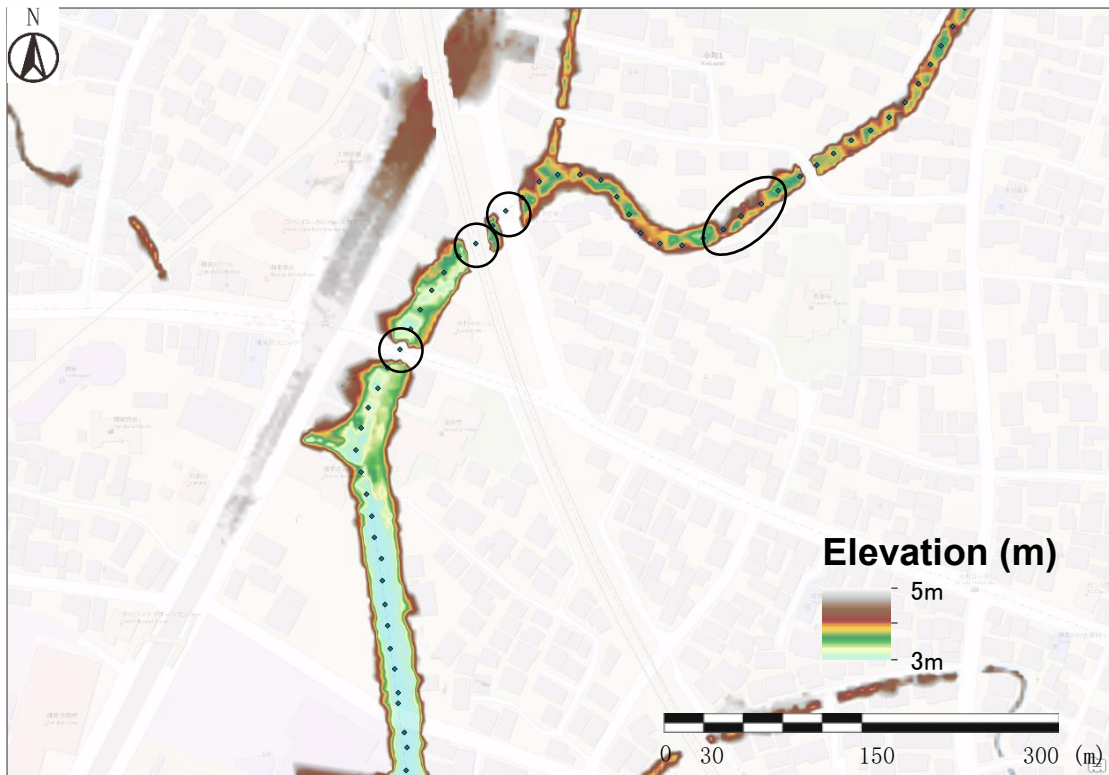
Figure 3-6C. The elevation color map of 840m-1300m. The circles indicate the points of bridges and roads which should be removed.
