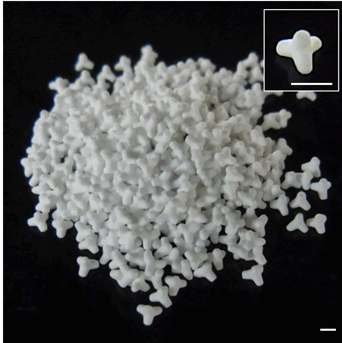
Fig. 1-1. Tetrabones® (TB) are tetrapod-shaped granular artificial bones made of \alpha TCP with the size of 1 mm. Scale bar = 1 mm.
