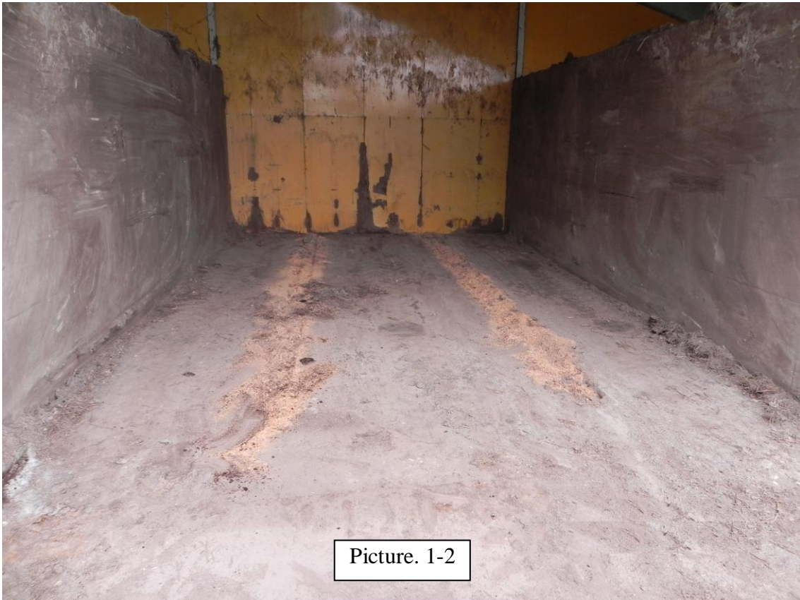
Picture. 1-2. The fermenter of aerobic ultra high temperature germentation for livestock waste. The size is 4.3 m wide, 7.3 m depth and 2.4 m high.
