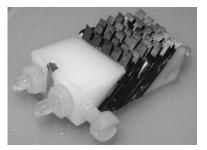
Figure 3.3: A tactile display using ICPFs, which are rectangular slices. Subjects wear it on the finger cushion of their index finger.
