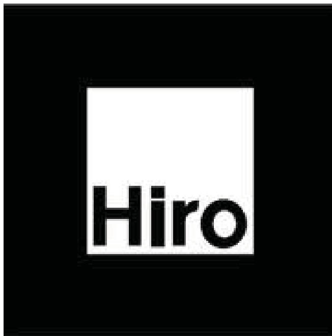
Figure 1.2: A typical marker in AR application. This is one of the sample markers in ARToolkit. ARToolkit is one of the first project in using the marker to make the easy registration for AR applications[17].
