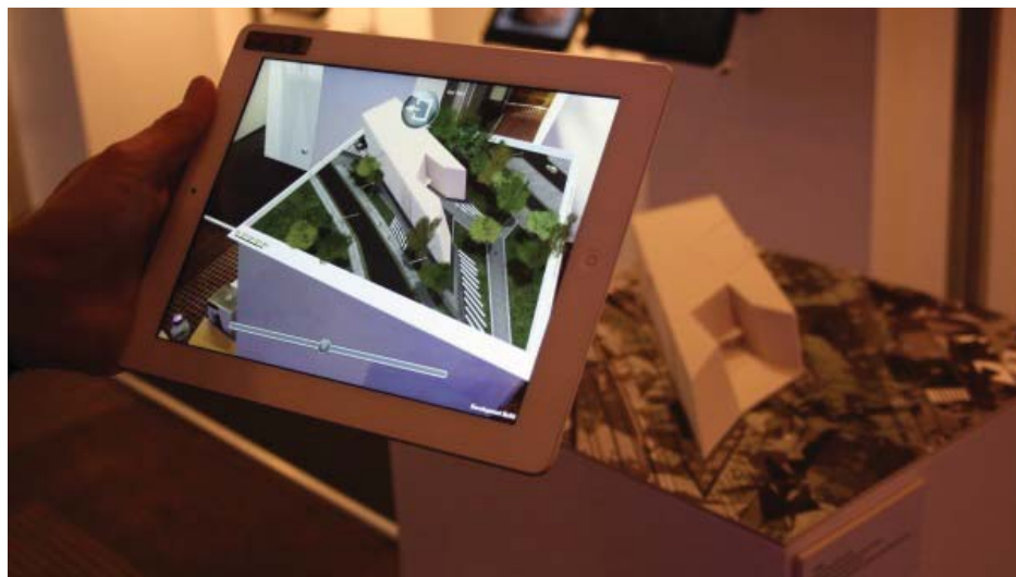
Figure 1.5: iPad-based augmented 3D-printing models. The 3D-printing model is used as a marker. The whole AR system was invented as a new way to show architectural plans[14].
