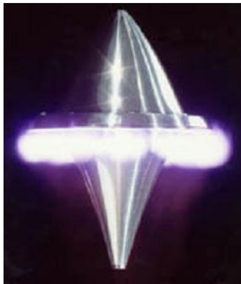
Figure 2.1. Shape of RP laser propulsion thruster
