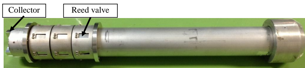
Figure 3.10. With reed valve type thruster (three pieces of reed valve part)
