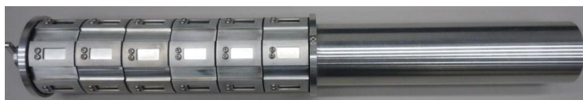
Figure 2.2. Shape of microwave rocket thruster
