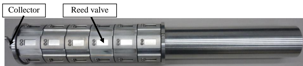
Figure 3.11. With reed valve type thruster (six pieces of reed valve part)
