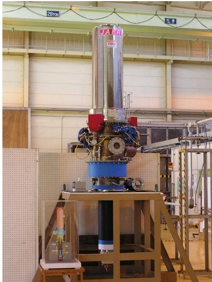
**Figure 1-5 Gyrotron**
