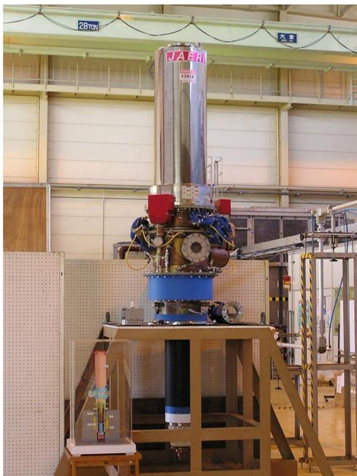
**Figure 1-5 Gyrotron**
