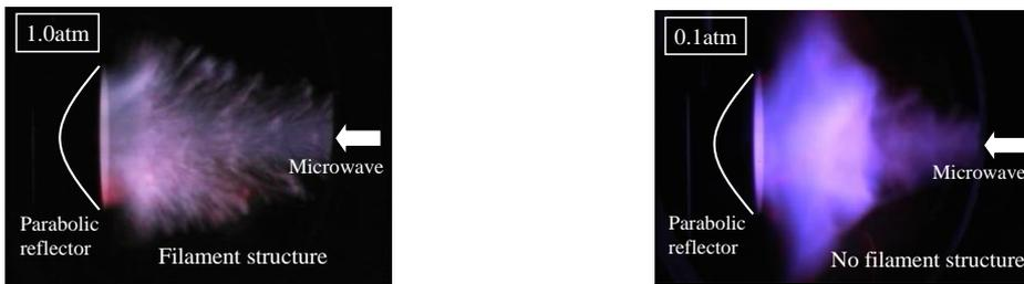
**Figure 1-1 Millimeter wave discharge in high and low pressure**
