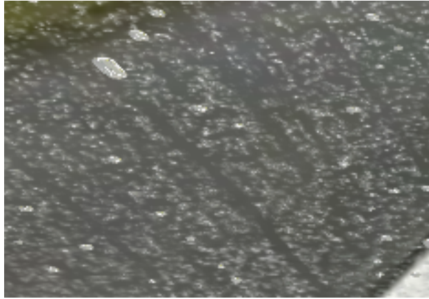
Figure 3.9: The Lotus effect. Small and still droplets are rendered as a normal map on the windshield. Large and moving droplets are rendered as pseudo-hemispheres.
