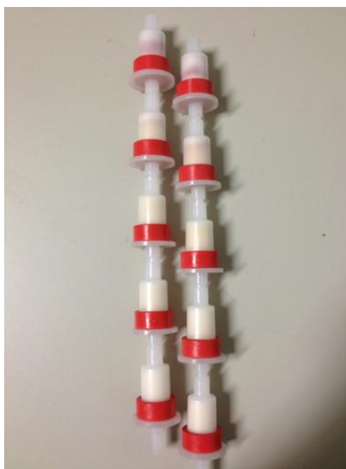
Figure 7 C18 SPE column
