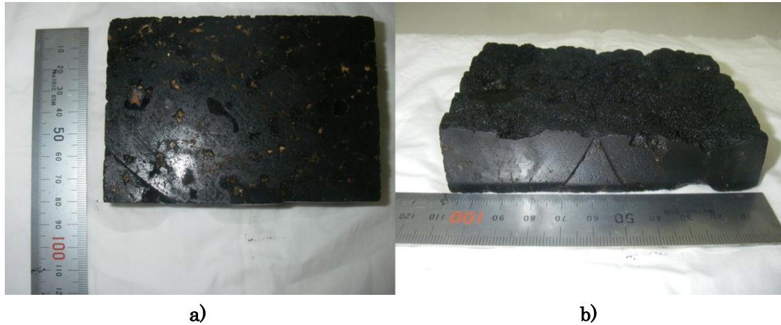
Fig. 2-7-1 a): a flat surface of manganese crust sample cut by rock cutter, b): a hubble surface maintained natural state(Surface 2).
