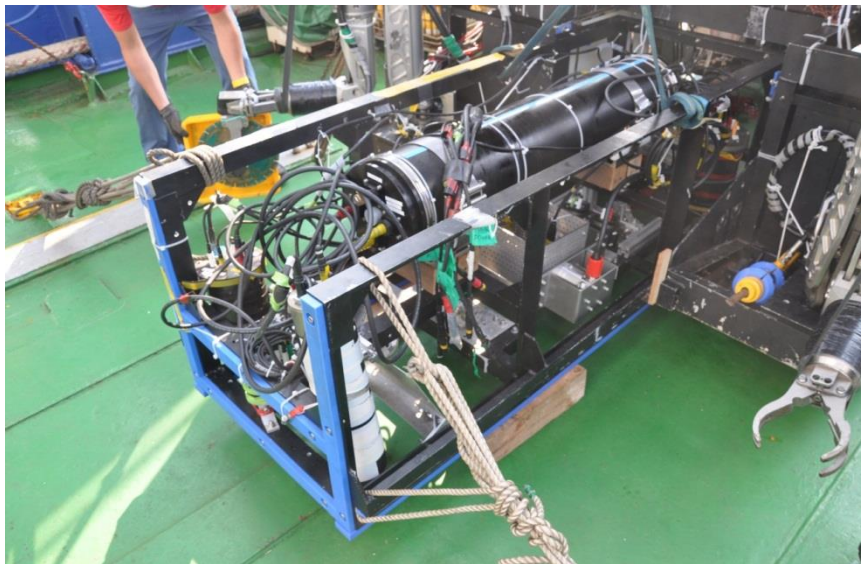
Fig. 5-1 Hyper Dolphin and payload skid with active gimbal system
