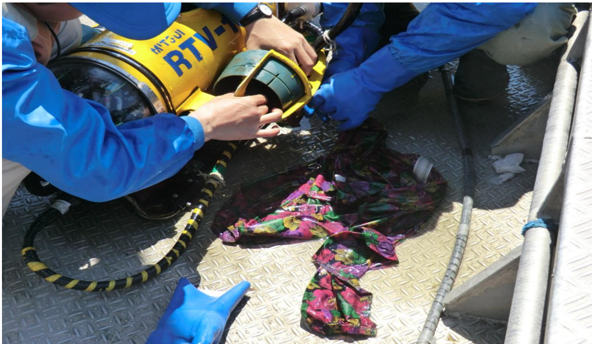
Figure 1.1 Floating objects got caught to thruster
